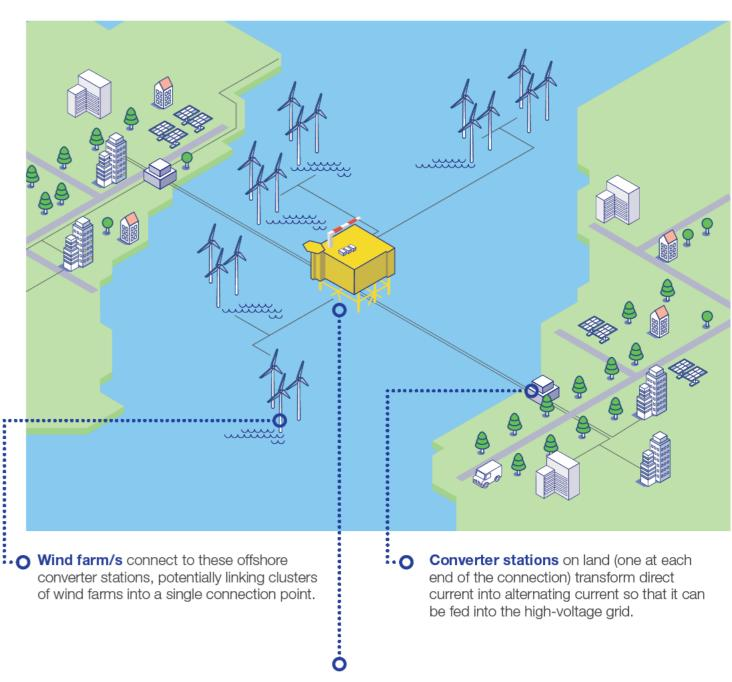
An **offshore converter** station transforms the alternating current into direct current, enabling it to pass through the HVDC cable.
