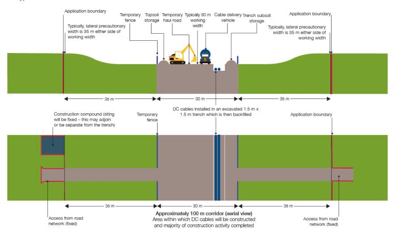
This illustration is for illustrative purposes only and is intended to show the typical construction of DC cables for interconnectors in the UK
